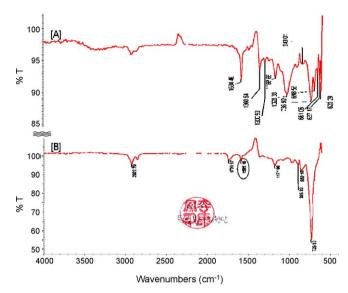
Fig. 3. Spectra of (A) a ballpoint pen and (B) a ballpoint pen on a seal ink.
