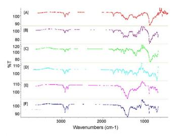
**Fig. 2.** Blind test result showing micro-ATR FTIR accurately matches unknown sealing paste after running queries in the spectral database. (A) Unknown seal ink sample; (B) a seal ink sample, S2 (match value = 79.19); (C) a seal ink sample, S4 (match value = 54.04); (D) a seal ink sample, S7 (match value = 39.18); (E) a seal ink sample, S3 (match value = 37.63); (F) a seal ink sample, S1 (match value = 37.23).
