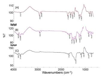
**Fig. 1.** Typical ATR FTIR spectra for seal inks of the same color but different manufacturer (A) a seal ink sample, S6 (B) a seal ink sample, S7 (C) a seal ink sample, S8. These IR spectra for seal inks stamped on white papers were subtracted with the IR spectrum of white paper.
